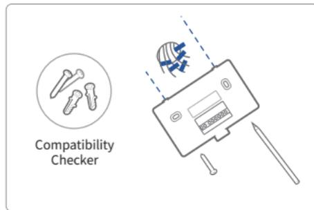
Use the picture you took before as reference to wire, the following chart is a wiring diagram for common systems, please make sure that a C-wire exists in your old thermostat system.
